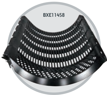
CORN, SOYBEANS MaxThresh™ in position 1 MaxRound™ in positions 2–6
